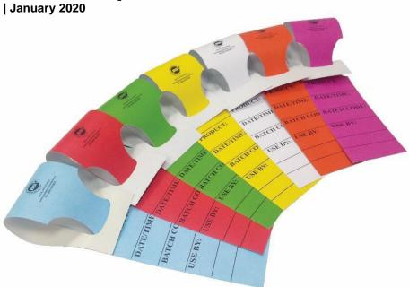
The metal detectable loop tags are designed to address foreign body contamination concerns associated with regular paper traceability tags used in food processing environments. Metal detectable loop tags contain a 7 micron thick layer of aluminium foil designed to trigger metal detection systems, even when the tag is shredded into small pieces.
